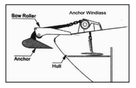
Mount on the top of the deck. Attach plywood under the deck to spray the force, if it is a aluminium, or fibre glass thinner than 6mm.
